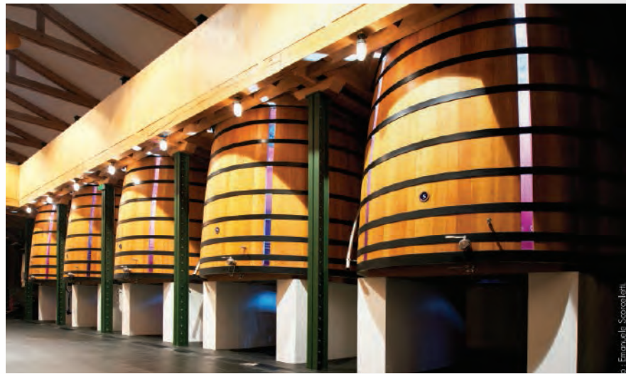
Seguin Moreau created tanks with transparent staves for Château Mouton Rothschild. The see-through staves allow winemakers to view fermentations in action.
